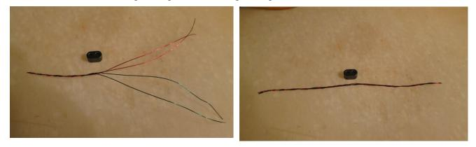
The end of this bundle that has the two loose crimped doubled ends is used to wind 4 turns through the core. I was careful to keep the windings adjacent as much as possible, not crossing over each other, to maximize the available space. A wood round pointed toothpick is useful to pack the windings to make space for the next pass. Be careful not to scrape the wire
