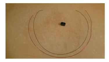
Bend each wire in half and crimp each bent end so it is flat.
