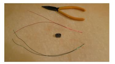
Twist the two doubled lengths together, making a single bundle of 4 wires.
