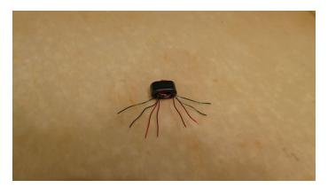
Then you connect up two wires to make one 8 turn center-tapped winding (using one color if you had two colors), then connect up the other two wires to make another 8T center-tapped winding. One of those becomes the secondary with its center tap used. The other one is the primary with no connection to the center tap.
