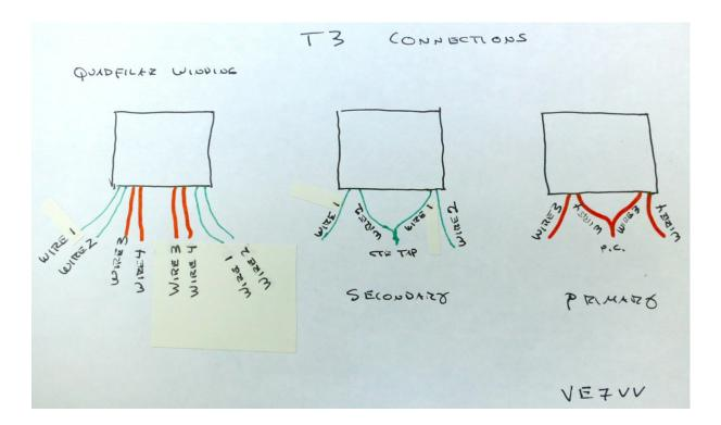
Use an Ohmmeter to make sure you connect up two *different* wires (Ohmmeter shows there is no connection).
